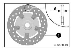
Check the thickness of the front and rear brake discs at multiple points on each brake disc to ensure it is at least thickness (A).
