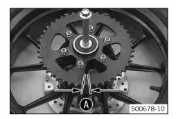
Lay the read wheel on a workbench with the rear sprocket facing upwards and insert the wheel spindle in the hub.
