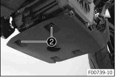
Mount and tighten screws **2**.
