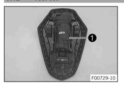
The tool set **1** is located under the passenger seat.
