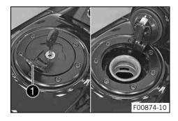
Lift the cover 1 of the filler cap and insert the ignition key in the lock.
