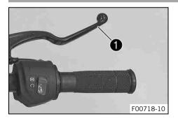
The hand brake lever **1** is fitted on the right side of the handlebar. The front brake is engaged using the hand brake lever.
