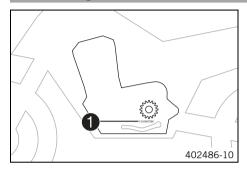
The engine number **1** is stamped on the left side of the engine under the engine sprocket.
