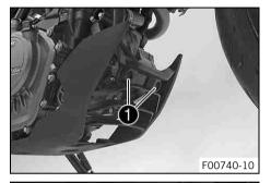
Position the front spoiler. Mount screws 1 but do not tighten yet.
