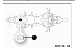
Diagnostics connector 1 is located under the passenger seat.
