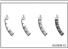
The coolant temperature indicator consists of bars. The more bars that light up, the hotter the coolant.
