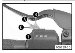
Light switch 1 is fitted on the left side of the handlebar.
