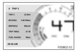
When the menu is closed, the  ${f Quick\ Selector\ 2}$  menu is opened by pressing the  ${f DOWN}$  button.
