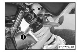
Adjust the spring pretension by turning adjusting ring ①.
