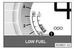
The fuel tank contents are shown in area 1 of the display.
